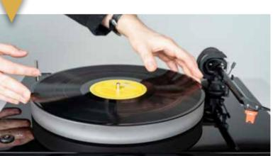
Carefully place the tonearm between platter and armrest and lower the tonearm lift.
