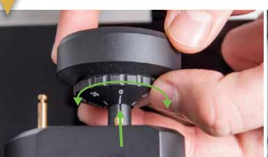
Turn the WHOLE counterweight counterclockwise until the scale reads 23.
