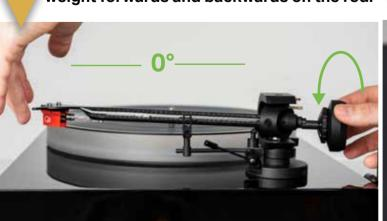
Hold the counterweight and set the dial to '0' by ONLY turning the dial to the marker.
